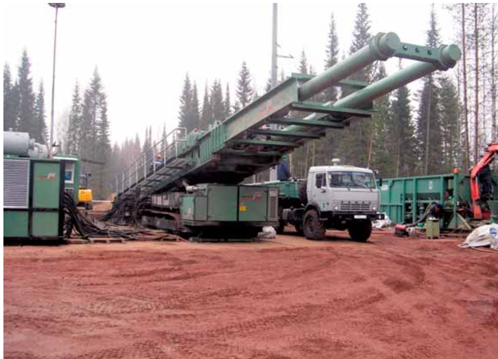
With its pulling force of 450t max. and a torque of 150 kNm, The Prime Drilling bore rig PD 450/150 AM is the horizontal drilling machine with the highest capacity in Russia.
